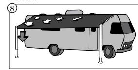
During light rain, lower end opposite from door to shed water and prevent pooling.
