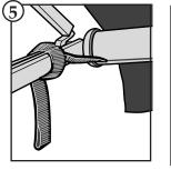
Slide one rafter arm up until it snaps Slide the pull strap to into place. Pull down and out on the right end of the the sliding rafter to remove slack tube, and wrap as from the fabric, and tighten the shown. black adjustment knob. Repeat for other side.
