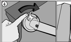
Grasp the pull strap, pull toward you, and flip the locking lever up to the ROLL UP position.
