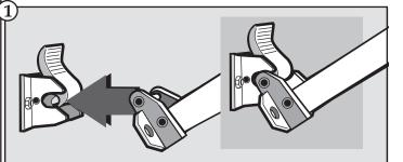
Pull stakes from the ground, lower arm to the shortest position, swing arm toward the vehicle, and snap the patio foot into the bracket. Repeat for other side and proceed to next step.
