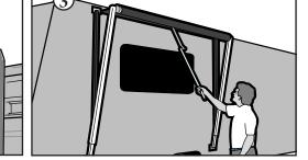
Hook the rod in loop, and pull all the way out.
