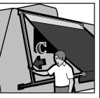
A: Loosen black adjustment knob. B: Lift slider catch. C: Slide the rafter arm down to the bottom of the main arm. Leave black adjustment knob loose. Repeat for other side.
